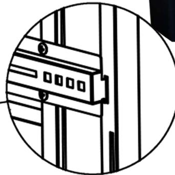
**Secure the horizontal beams with M5 bolts (plastic bag #8).**
