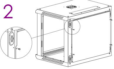
Install the brush type cable entries using M6 bolts/nuts. 2 bolts/nuts for each cable entry. Plastic bag #2.
