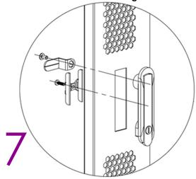
Use the plastic bushings (or, adjustable washers if needed) when mounting the front door.
