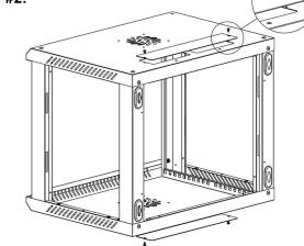
Using the plastic bag #2, or hardware set install the vertical mounting rails. The distance between the rails is to be determined based on the depth of the equipment or, the supplied shelves.
