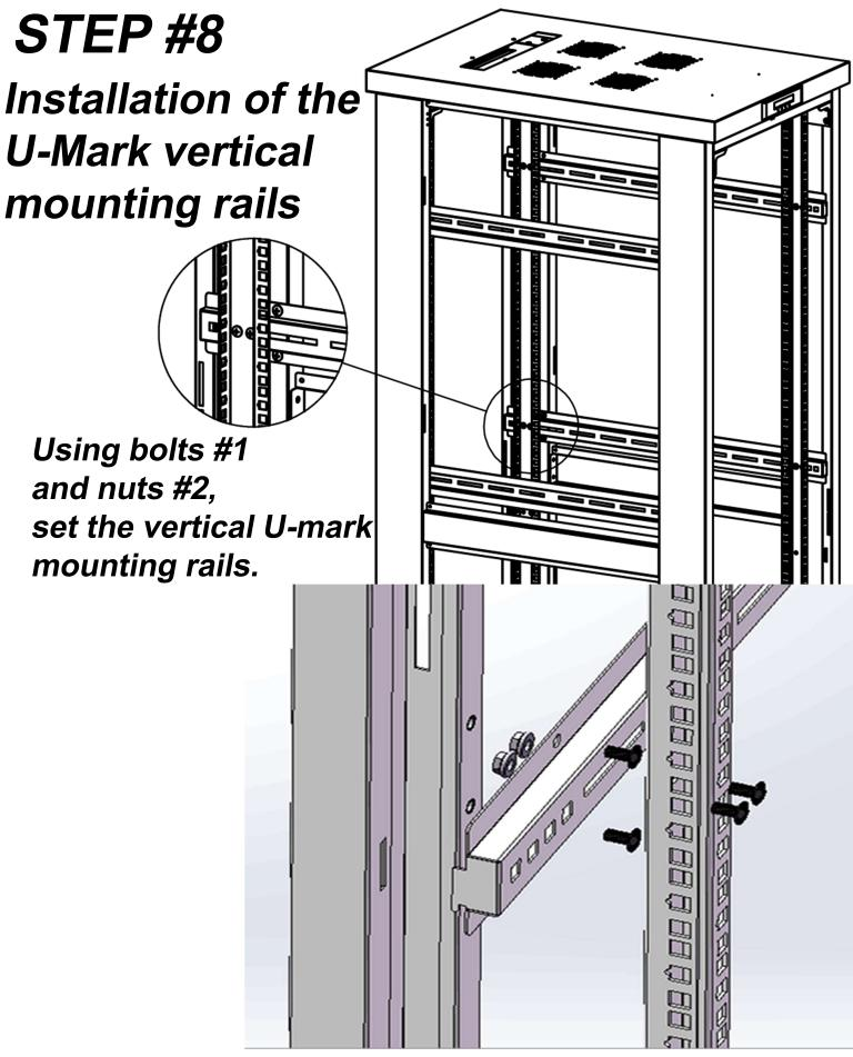
III The distance between the vertical rails is to be determined in advance based on the mounting equipment (or, the depth of the supplied fixed shelf)
