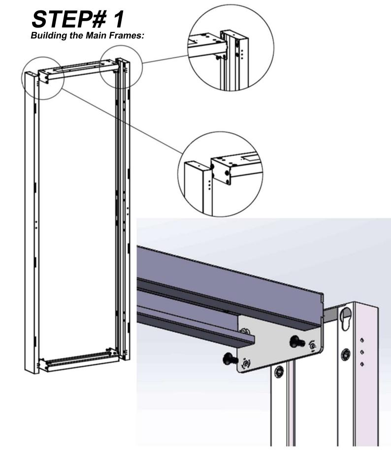
Combine the Horizontal (package 5/5) and Vertical (package 1/5) frame parts into one single carcass. Secure each connection with 2 X M5 bolts (plastic bag #8).
