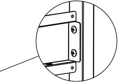
Using the bolts # 1, nuts # 2, install the intermediate horizontal side panels supporting beams on each side.
